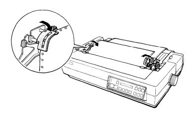
9. See that the paper is not crooked or wrinkled and lock the sprocket units in place.
